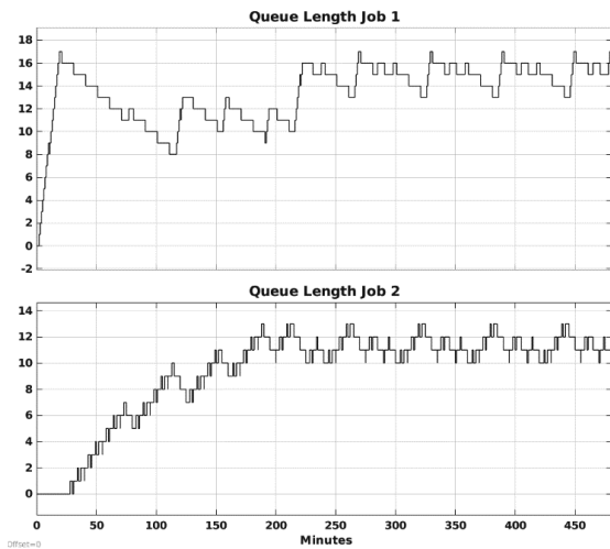
Figure 8. Time trajectories of the queue lengths computed using the learned strategy of a self-implemented Q-agent after 5000 episodes.
