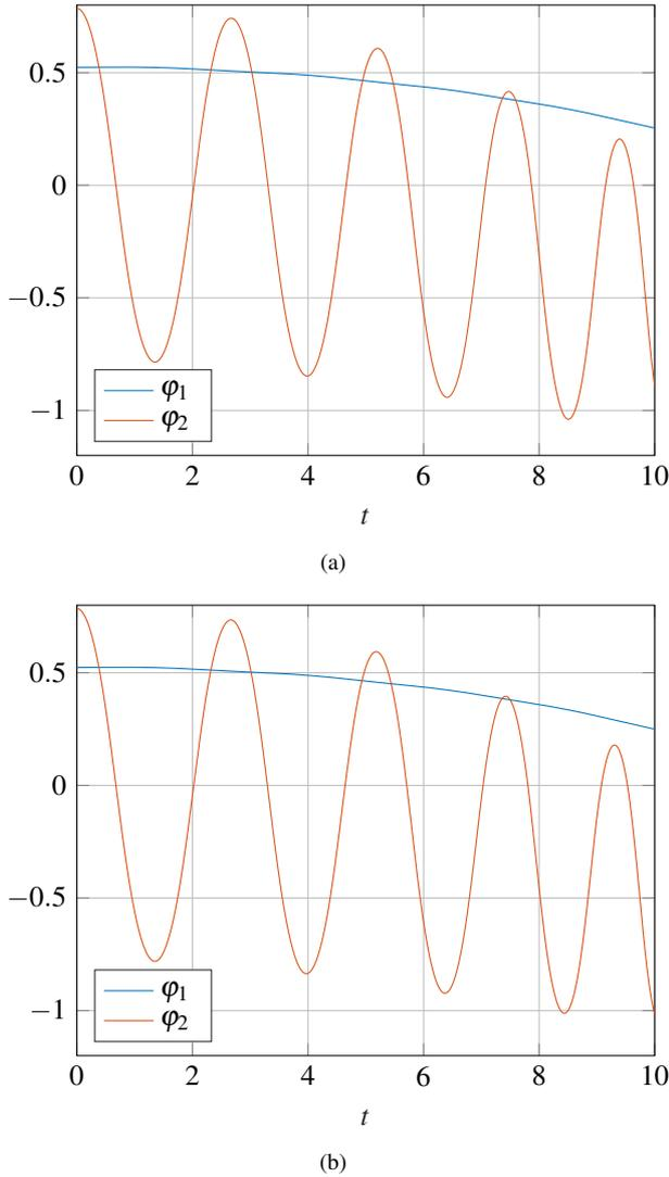
**Figure 4:** (a) Simulation with explicit Euler method, with step size  $h = 0.001$ , (b) Simulation with Heun method, with step size  $h = 0.01$ . Time plot of angular position. Both with simulation time 10s.
