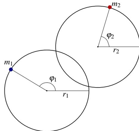
**Figure 2:** A sketch of the system setup, the blue dot represents the point mass  $m_1$  and the red dot the point mass  $m_2$ . Movement occurs in circular paths, with position vectors  $\varphi_1$  and  $\varphi_2$ , both with fixed radius  $r_{1,2}$ .
