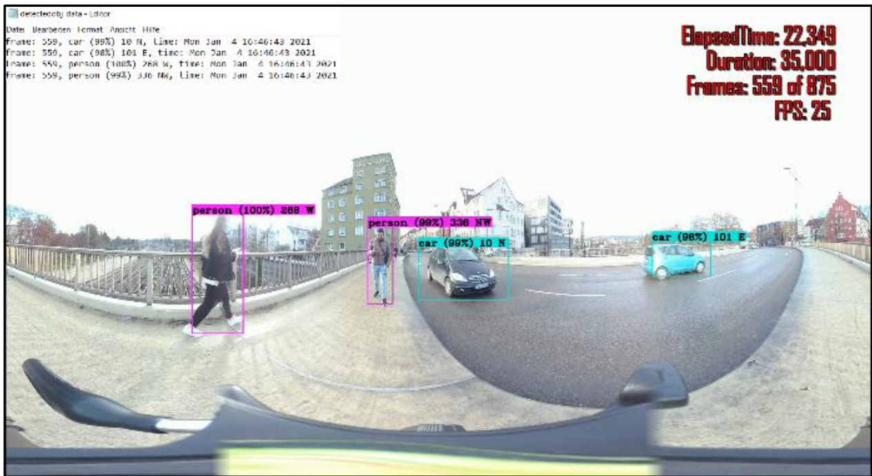
Figure 4: Object detection using the YOLO algorithm extended with an angle of arrival.
