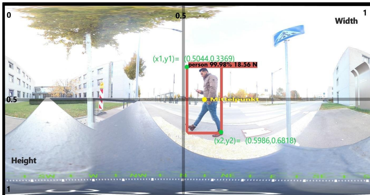
Figure 3: Example of the object detection extended with an angle of arrival.
